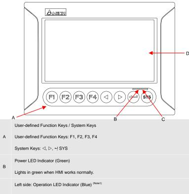
С The operation LED indicator blinks in blue when either the communication is carried out or the
